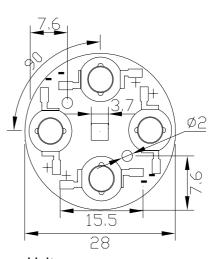
Unit: mm Tolerance:+0.3mm
